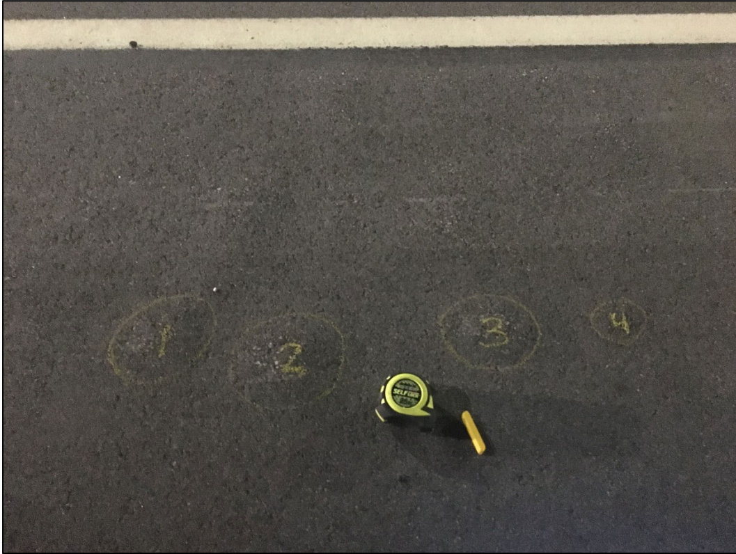
Figure 4. Photograph of group of 4 blisters evaluated with point-by-point IE and SASW testing in the eastbound right shoulder.
