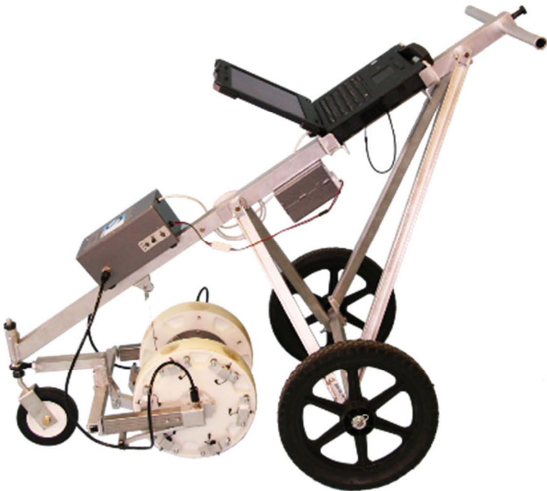
Figure 16. Sonic Surface Scanner (S 3 ) for slow-rolling Impact Echo (and Surface Waves) Scanning of Concrete Decks/Slabs and Asphalt Pavements with tests every 6 inches – note solenoid impactors on sides of sensor wheels and brass displacement transducers on wheel surface that are offset 30 degrees for alternating IE tests on the left and right wheels as it is rolled along.
